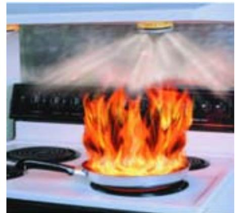
When a stovetop blaze touches the bottom of the FireStop®, a small pyrotechnic opens the petals of the can, and dumps out bicarbonate of soda to smother the fire in the pan. As it is deployed, the FireStop® also sends out a 146 decibel alarm.
